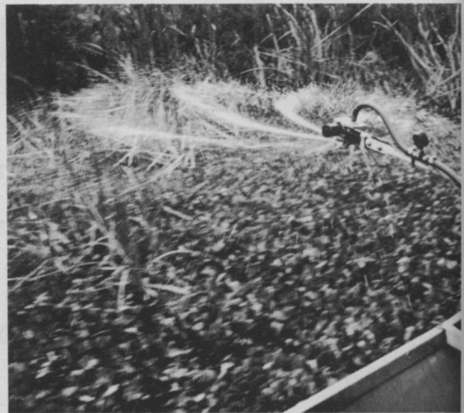
Directa Sprayer in action. Notice that the spray pattern is "wheel" shaped. Herbicide passes through the control box to the hub of the unit where it enters eight tubes which make up the delivery section. Nozzles may be attached to the tubes.
