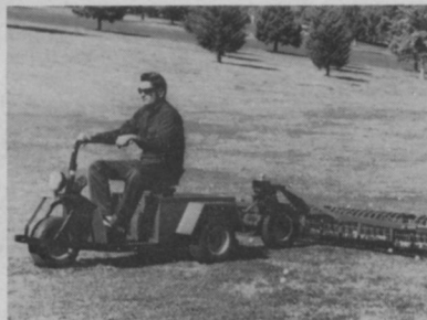
Hauling a 3-gang ball picker. Easily tows up to 250 lbs. of tools, chemicals, spikers, trash containers, and other equipment.
