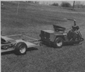
Low cost, low-bed utility trailer with big 35" x 66" bed, available as optional equipment.
