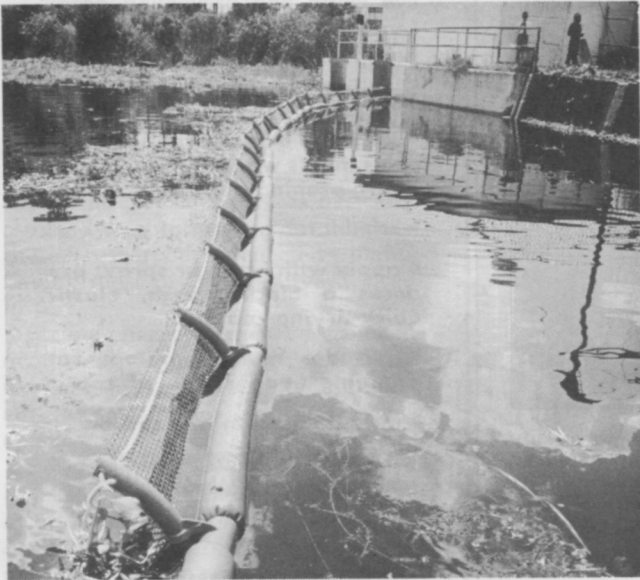
N-BAR FLOATING BARRIER SYSTEM: Sea Guard, Inc., New Castle, Del.
