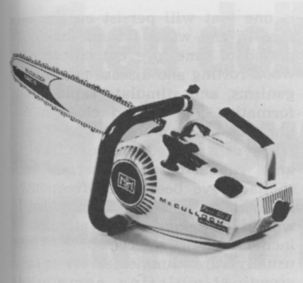
McCulloch Power Mac 6 is a good example of compact wrap-around styling and well-grouped controls.
