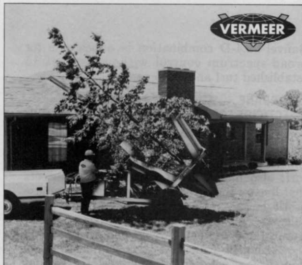
"Instant Shade!" Popular Vermeer Model TS-44A transplants a big 4" diameter tree in minutes! Four hydraulically-operated, high-tensile steel spades form maximum size tree ball 42" diameter, 46" deep... lift and transport trees with absolutely no hand labor required.
