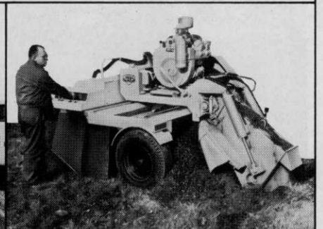
MODELS 2436 AND 2460 — Vermeer's new "reach-out" models cut wider, closer and faster. Low silhouette design. Cuts 24" deep, with 36 or 60 hp engine.
