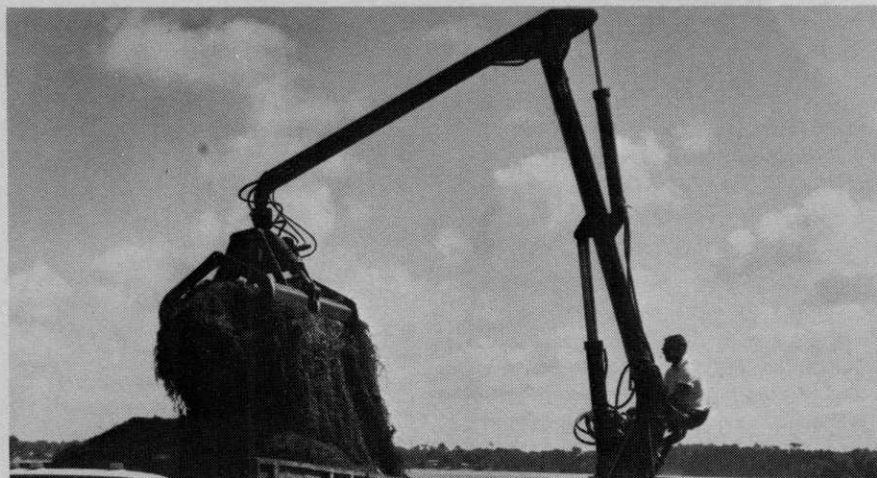
Sheer volume is a major problem with mechanical harvesting of aquatic weeds.
