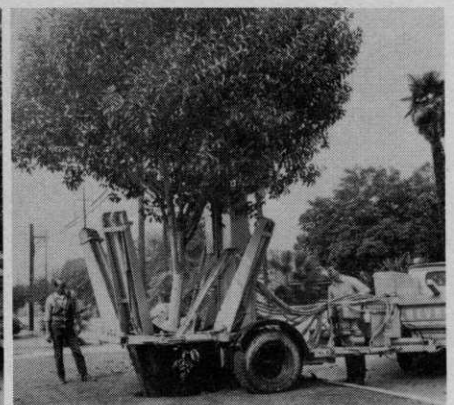
Trailer-mounted Vermeer model TS-44A, above, gently lowers large tree into previously dug hole. Instant shade . . . in minutes!
