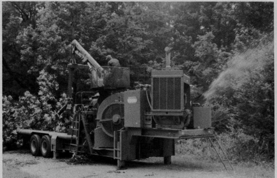
Heavy duty articulated knuckle boom loader with 20-foot reach and 400 degree swing along with powered crushing rolls constitute the heart of Precision Chipper's new Tree Destroyer.
