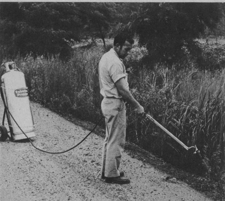
Suburban Propane has two basic equipment plans. One is a three-foot torch and 100 lb. cylinder mounted on a cart for intermittent light to medium flaming. The other is a
