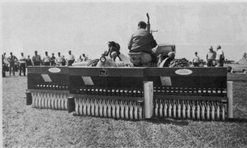
Wide-swath coverage in seeding and fertilizing was the feature of this equipment shown and demonstrated at the American Sod Producers Association. The spreader at left, distributed by O. M. Scott & Sons, Marysville, Ohio, lays down a strip of fertilizer about 30 feet wide. Jacobsen Manufacturing Co., has ganged the Rogers Seeder it bought recently and offers hydraulic lift capability for turn-around and transporting.
