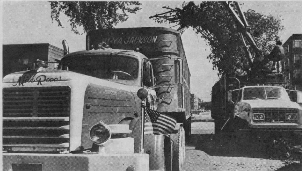
Chicago has expedited its tree removal operations by using clam-type loaders and trailer transport trucks leased from area commercial tree companies. This truck is owned by Jackson Tree Service.
