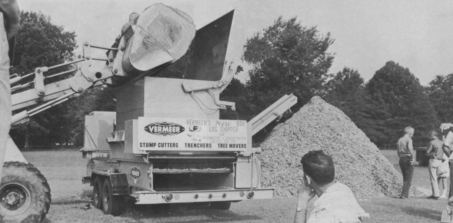
Vermeer's 604 log chipper is designed to take tree sections six feet long and up to 4 ft. in diameter.
