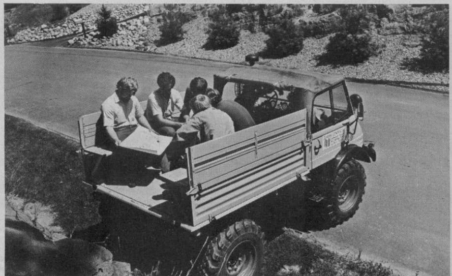
The Unimog can be loaded with crews and equipment and, if necessary, can tow a trailer. Top speed is 47 miles per hour.
