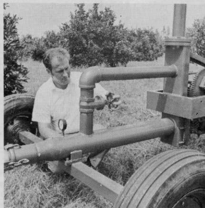
Forward movement of the Turbo-Rain can be adjusted with this by-pass valve. The valve regulates the amount of water passing through the turbine, thus changing the "walking" speed of the machine.
