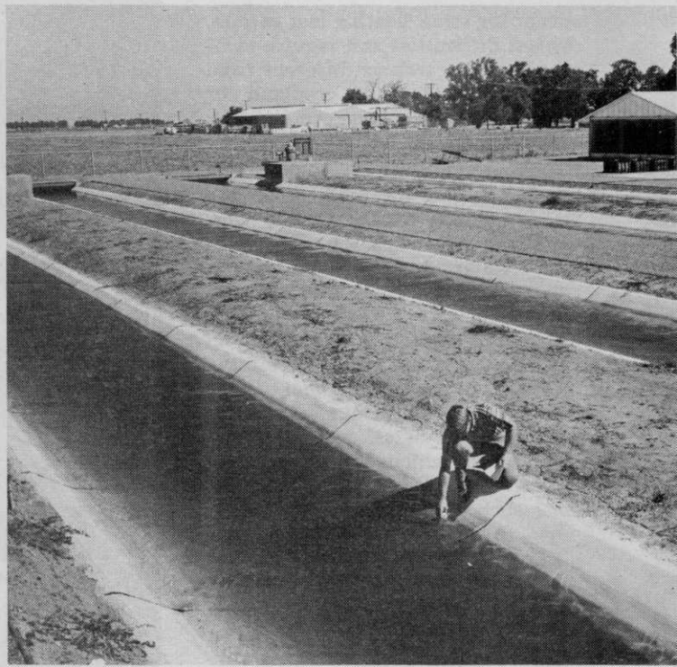
have shown promise for control of submersed weeds or algae in static water tests. Then initial field tests are conducted in four concrete-lined, 150x15x3-foot canals. The experiments determine the effects of herbicides on different species of submersed weeds, and on fish and Asiatic clams. Photos by California Department of Water Resources.
