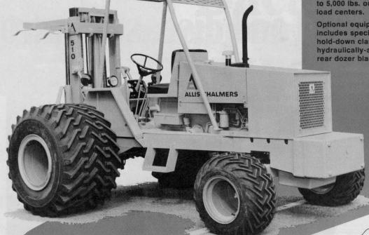
A hand/foot oil-type reverser speeds up cycle time-gives your operator precision control at any speed whether going forward or in reverse.
