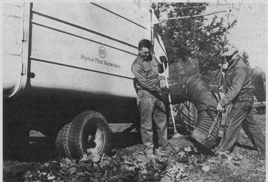
Southern Illinois University, Carbondale, has cut leaf-raking time in half with a vacuum leaf collector that swoops up 14 square yards of leaves per load and grinds them to mulch. James Mayer, left, and Homer Pinkerton, physical plant workmen, operate the collector. The mulch, formerly burned, goes into a compost heap for campus use.
