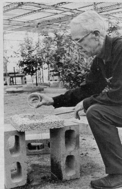
Dr. Sterling Richards, University of California scientist at Riverside, shows how easily water goes through porous block mulch he invented. Used around trees or other plants, blocks reduce water loss, soil compaction, salt buildup, and weed growth. UC has obtained a U. S. patent and has control of commercial license agreements.
