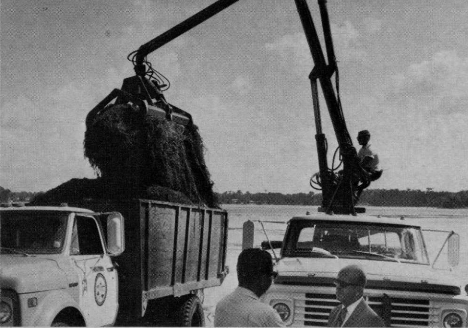
The Prentice loader will transfer a harvester load of weeds to a truck in about three 1,000-lb. bites. In the foreground, Andy Price, Pennwalt Corporation aquatic biologist, visits with Jay Blanchard, Winter Park's director of parks and recreation.
