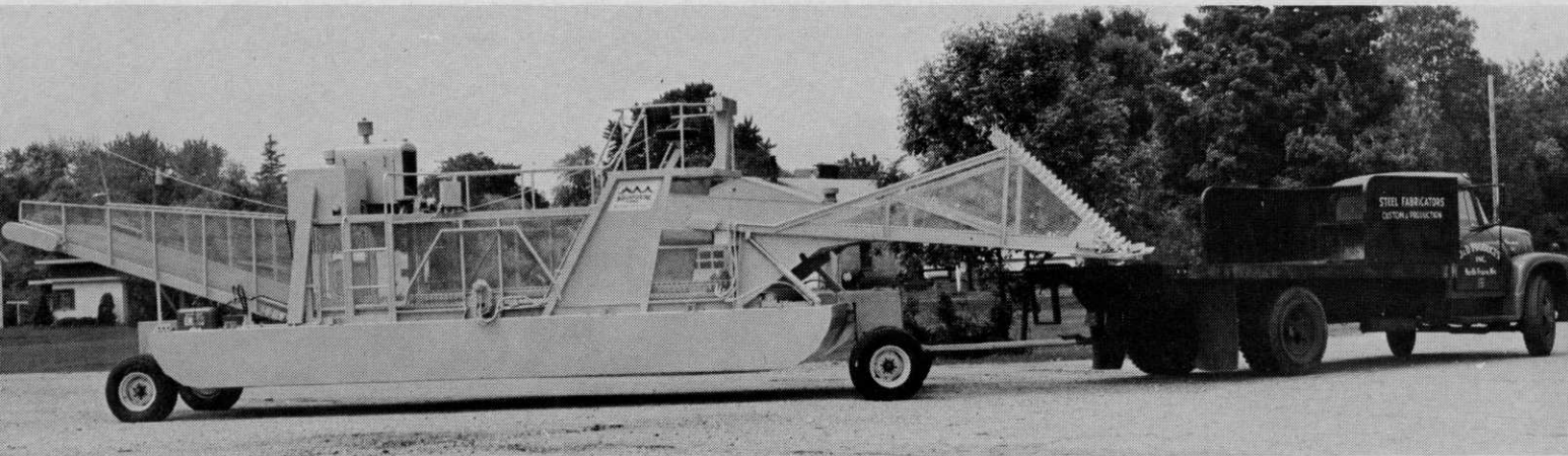
Attachable wheels connect easily to the H-650 Harvester, making it quickly mobile. It's easily towed with a minimum loss of cutting time.
