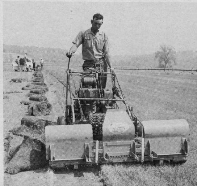
Princeton Turf of KC harvests sod with Ryan cutting and rolling equipment. An elevator loads bigger trucks.
