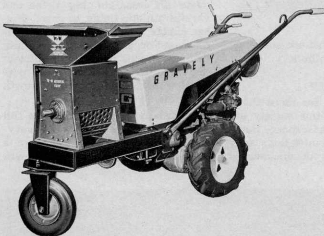
W-W Grinder Corporation offers a shredder that can be powered by a garden tractor with the use of a V-belt pulley. A stabilizer bar is provided which is simply and easily attached to most garden tractors. This Model 5 unit provides up to six yards per hour capacity.
