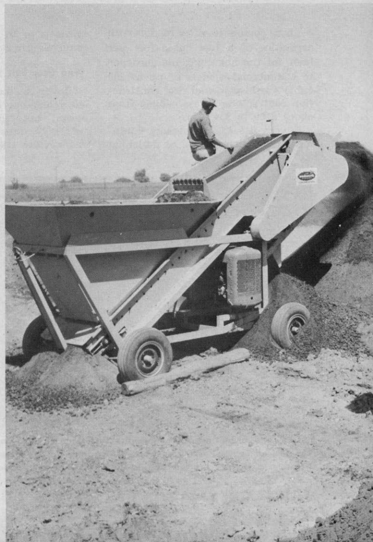
W-W Grinder Corporation offers a shredder that can be powered by a garden tractor with the use of a V-belt pulley. A stabilizer bar is provided which is simply and easily attached to most garden tractors. This Model 5 unit provides up to six yards per hour capacity.
