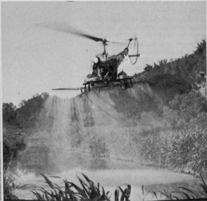
Invert emulsion enables ROWCO pilots to target herbicides on water or right-of-way from up to 75 feet in the air and still control pesticide drift.
