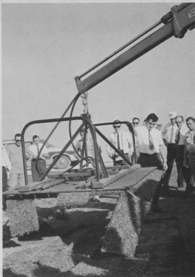
Automatic sod pick-up, 54"x96", manufactured by Stanco Midwest Sales, Inc., Chicago, Ill., was demonstrated at Ousley farm during tour.
