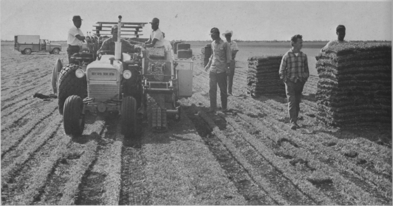
Nunes sod harvester in operation at Resmondo farm, first tour stop made by growers. Some 1300 acres of sod is grown yearly in this operation.
