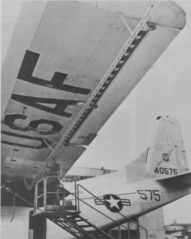
Spray boom is being installed on wing of twin-engine UC-123 used by the 'Ranch' for defoliation missions.
