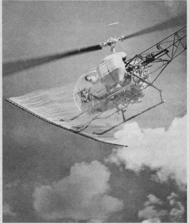
Microfoil properly trimmed in flight produces pattern above with appearance of a white sheet. Shot taken at Winter Park, Fla.
