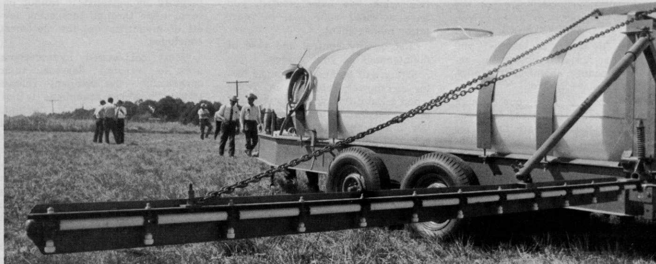
The talking point for this 1,000-gal. spray tank is its baffle construction. The two halves are molded separately then sealed together in tongue-and-groove fashion, adding strength, say Red Ewald, Inc., representatives. The spray rig comes with 100 feet of hose. The company is headquartered at Karnes City, Tex.
