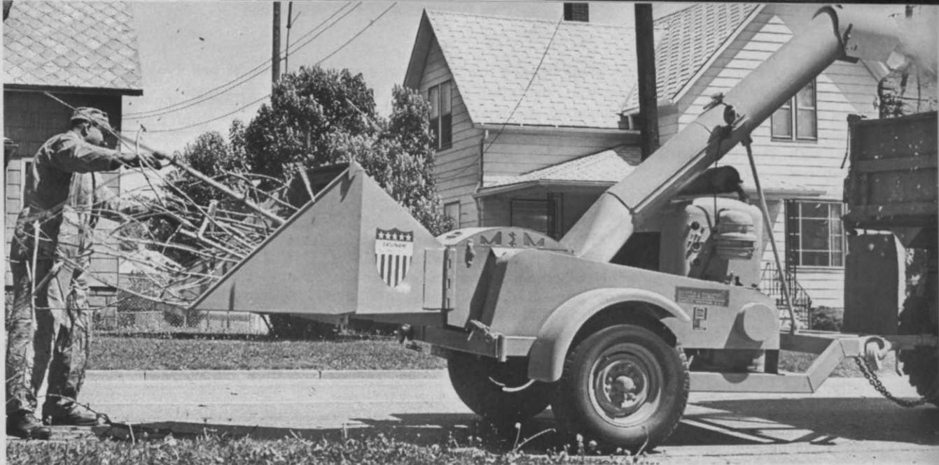
City-owned brush chippers—like this one of the City of Saginaw, Mich., 1969 All-America City—increase the efficiency and decrease the cost of free removal and pruning. Chips are frequently used as mulch for golf courses, parks and zoos.
