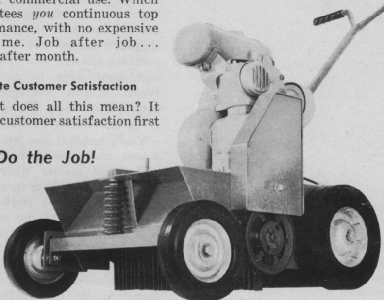
Simple, Efficient Height Adjustment Raises or Lowers the Rotor to Fit the Job.
