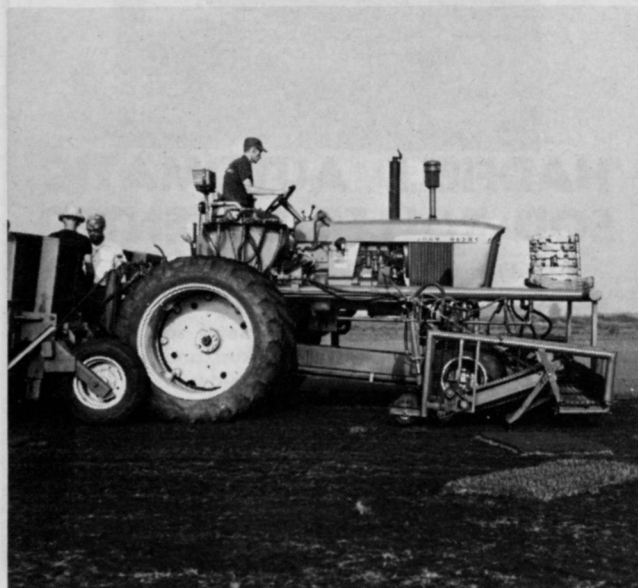
Side view of Don Morrill's sod harvester. Unit is designed to roll sod for pallets.
