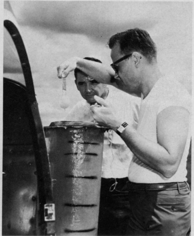
Perdue looks on as Charles J. Fox, technical representative of Hercules, Charlotte, N. C., makes viscosity test of Vis-ko-Rhap.
