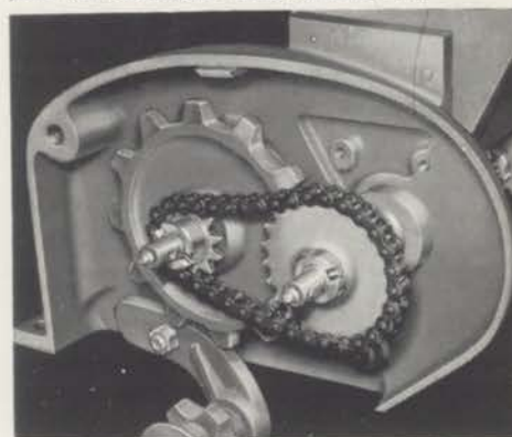
SPROCKETS afford a dual range of seeding rates. Small sprocket on driver shaft (shown) is for lighter seeding. For heavier rate seeding, you simply reverse the mounting of the sprockets.
