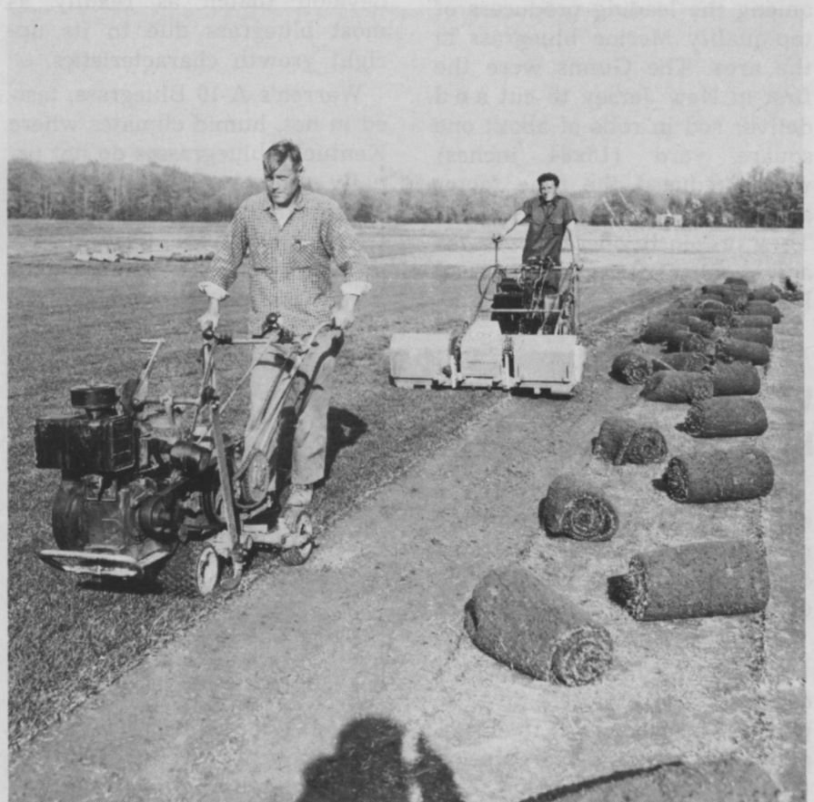
With early spring sod care problems solved, cutting and rolling good sod is relatively simple, according to Gunn. Sod is cut 16" x 84" with Ryan cutter and rolled with Ryan roller.
