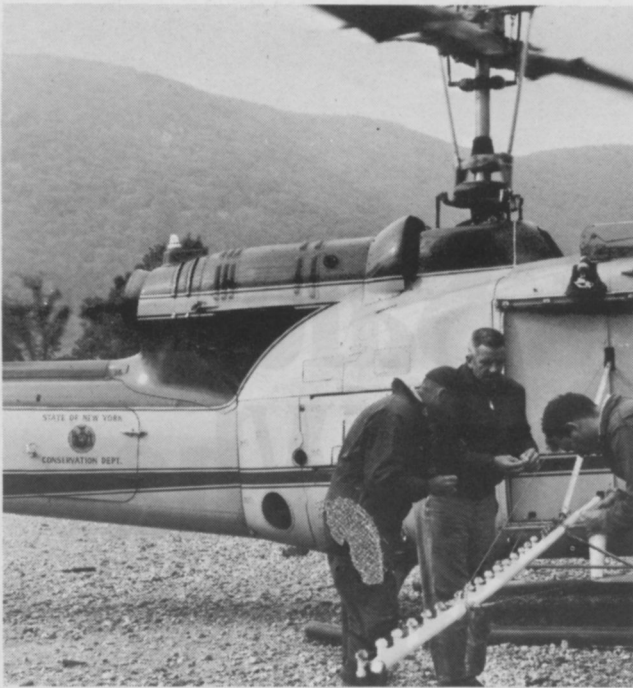
Spray nozzles on helicopter spray rig are cleaned and adjusted prior to loading with insecticide.
