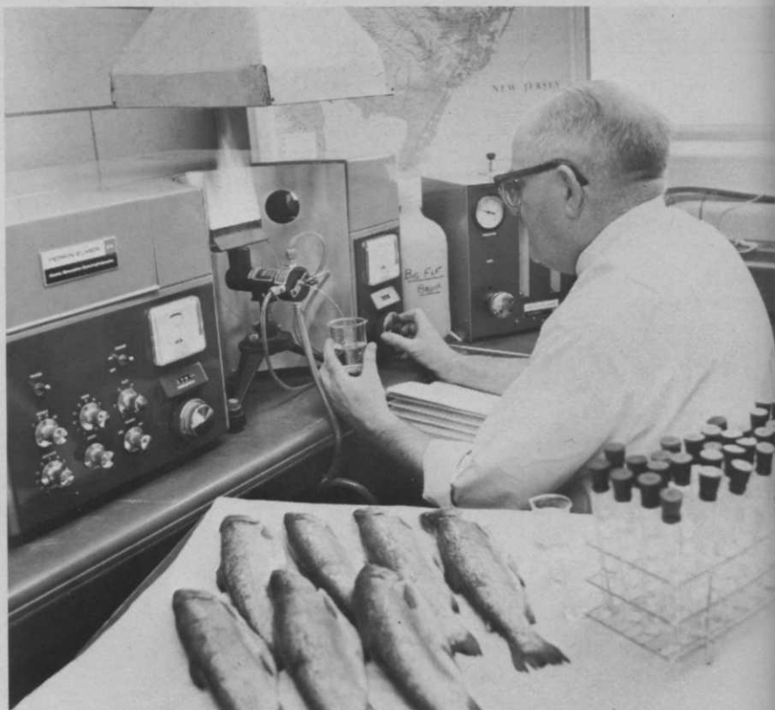
Dr. Stephen J. Toth, Soil Chemist, Rutgers University, uses a Perkin-Elmer Model 303 Atomic Absorption Spectrophotometer which determines the content of metallic elements in water samples down to parts per million level.
