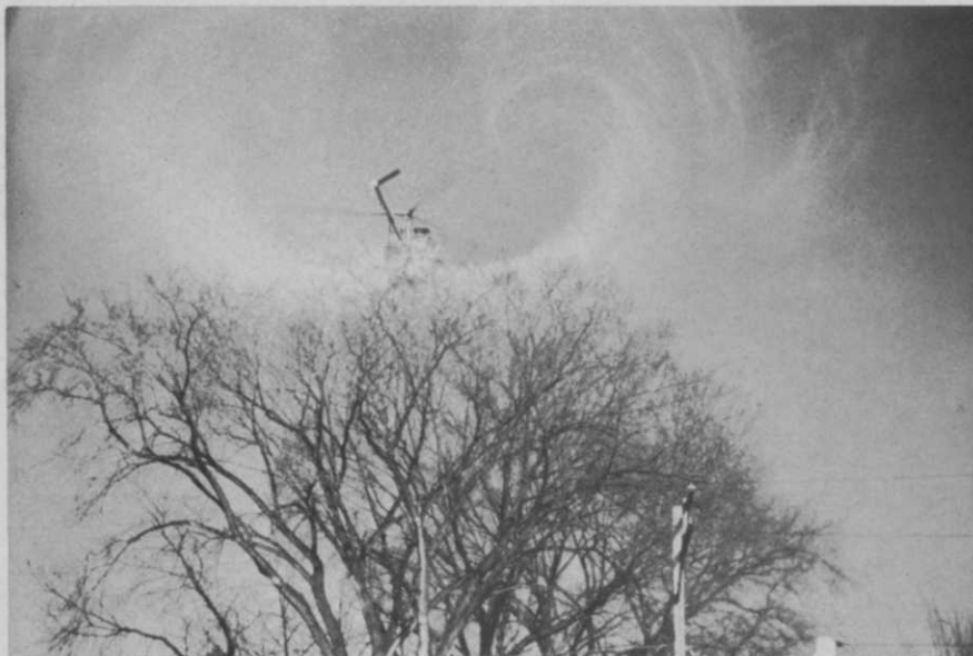
Aerodynamic characteristics of the helicopter's rotor system creates what is referred to as "blade tip vortices." Because of the extreme turbulent air created, vortices are normally considered an undesirable area in which to introduce spray. Experience of pilot along with spray equipment thus become very important in even coverage. DuPont depends on vortex action to increase coverage in hard-to-cover tree tops and crotches.
