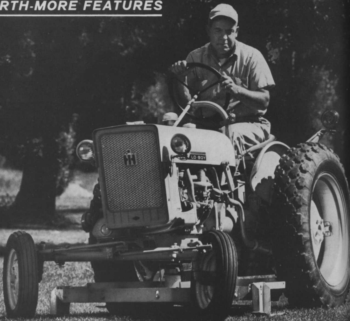
CUB LO-BOY with 60" center-mounted rotary mower.
