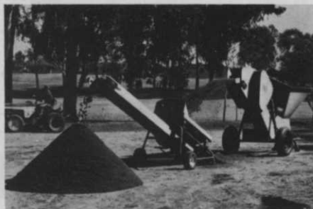
Superintendent 120 and POWERscreen ideally suited for preparation of topdressing and minor construction and repair jobs.
