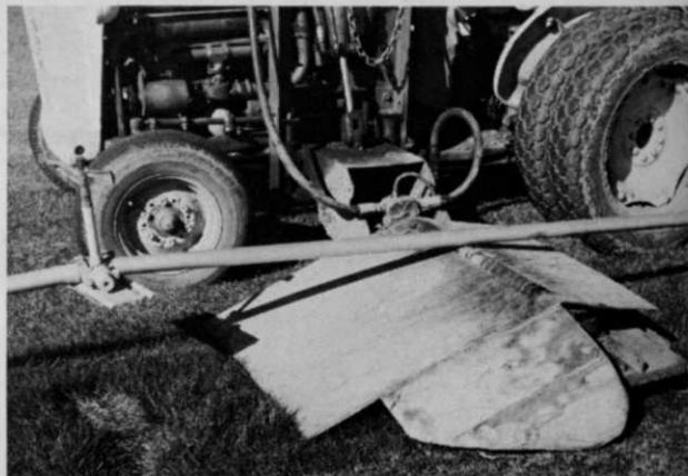
Close-up of shielded rotary mower in operation under Green Valley irrigation pipe.
