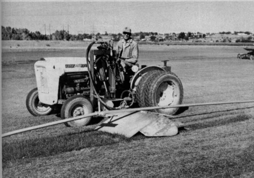
Longtime employee Tony Nickerson does most of mowing for Green Valley. Equipment consists of a diesel-powered 7-gang mower with this supplemental custom-built rotary unit.
