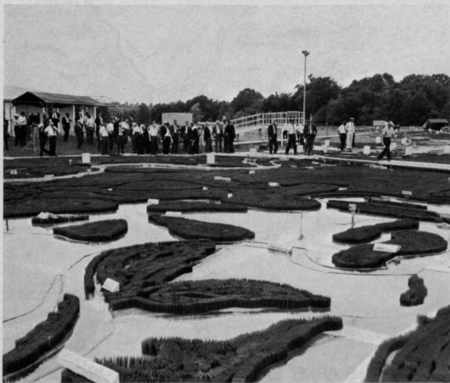
Scale model of Mississippi River and its tributaries shows visitors at the Waterways Experiment Station how the flood control operation works.
