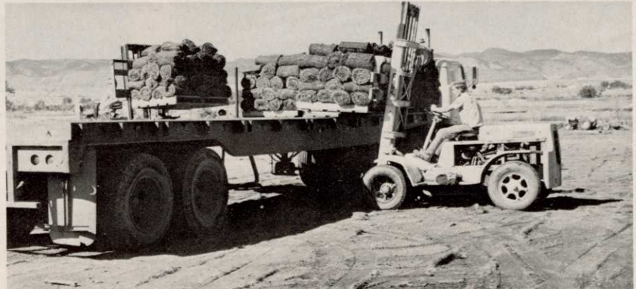
Once sod is palletted, fork lifts are used to quickly load trailer trucks. Loaded trucks are covered with a tarpaulin to protect sod from sun during transport. Tarp also helps hold sod rolls in place on pallets.
