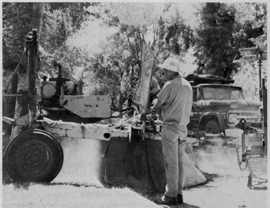
Operator removes last traces of stump in residential area with Vermeer stump machine. In this particular instance, stump is from large sycamore tree which was victim of anthracnose.
