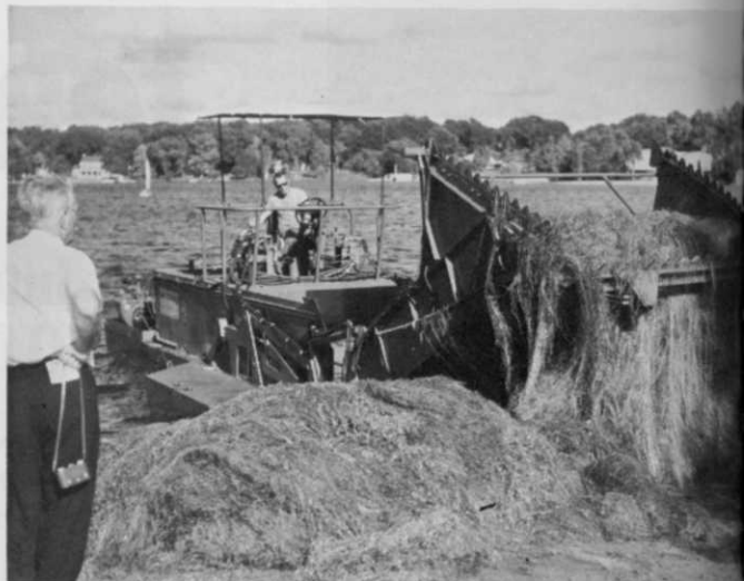
Mechanical harvester at right is owned by city of Winter Park, Fla., and is used to harvest aquatics as a means of keeping lake open for recreational purposes.
