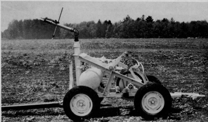
Automatic self-propelled irrigation sprinkler which is new on market delivers up to 550 gpm with diameter range up to 425 feet.
