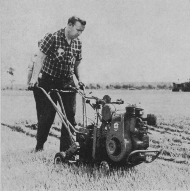
Ryan sod cutter is used to cut sand soil-based sod into 1'x2'x1" strips for loading on pallets. Checking out cutter is David Pipkins, field foreman.
