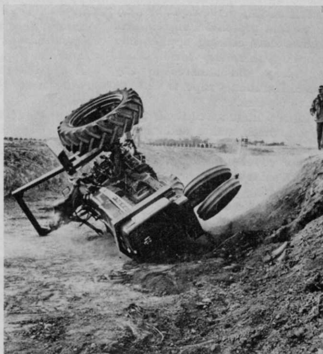
Protective frame in this test protects dummy, but in regular operation would likely prevent serious injury or death to operator.
