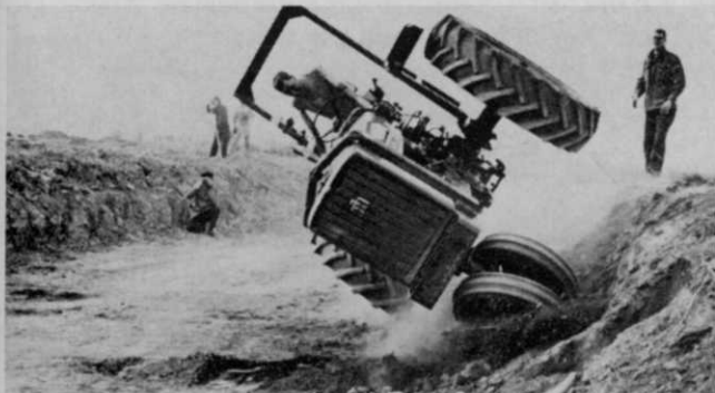
Without safety bar tractor operator would be helpless.
