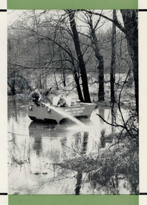
Cargo capacity of 1400 pounds and amphibious capabilities make Swamp Spryte with Myers sprayer essential equipment in treatment of shallow, swampy areas in New Jersey. See article on pg. 16.
