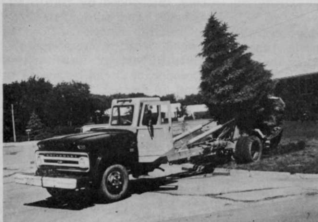
Vermeer's truck-mounted tree mover speeds hydraulic lifting and replanting of trees up to 7 in. to 8 in. in diameter.
