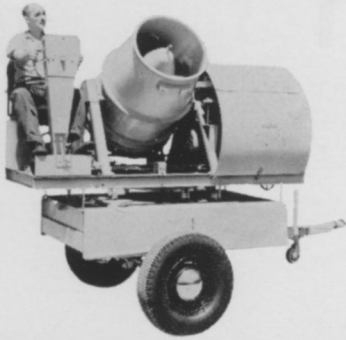
MODEL 100G ROTOMIST® shade tree, sanitation, mosquito control, leaf windrowing. 29" fan delivers 28,000 CFM at 100 mph.
