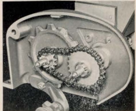
SPROCKETS afford a dual range of seeding rates. Small sprocket on driver shaft (shown) is for lighter seeding. For heavier rate seeding, you simply reverse the mounting of the sprockets.
