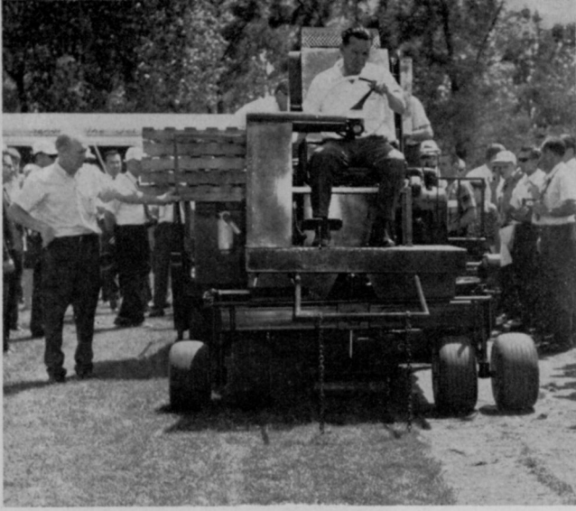
Princeton Turf Farms' Sod Harvester is capable of handling up to 10,000 square feet of cut and palletized sod per hour, based on report during field day demonstration. Wiley Miner, president of Princeton Turf Farms, on hand for the field day, was instrumental in development of the machine which operates with 3 men and produces uniform pads of folded sod, stacked on pallets.
