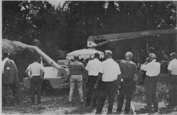
Pitman chipper built by Pitman Manufacturing Co., Grandview, Mo., features according to the maker, shallow cutting action, unique self-aligning cutting blade and emergency safety brake.
