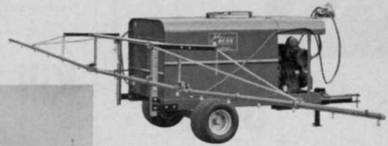
TURFKEEPER handles high pressure spraying applications of liquid fertilizer, weed or brush control chemicals. 17-nozzle, 3-section boom, wide flotation tires.
