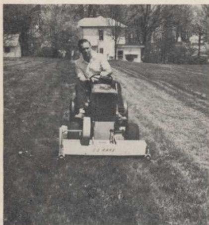
Thatch removal was part of the bluegrass test; here performed with an attachment to the John Deere garden tractor.
